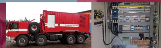
→ FH Bohunice Brno - building „CH“ Genset 860kVA, EuroSilent
